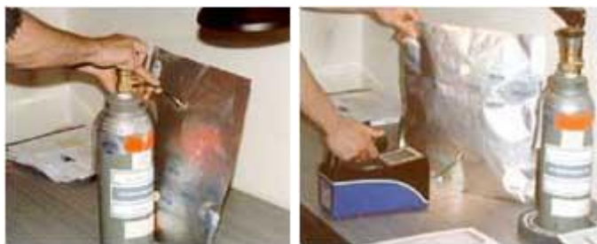
On site fast calibration of PID and IR channels
